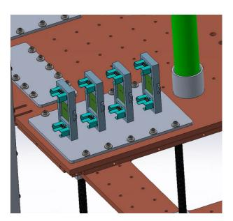
64 Channels in Cryostat
