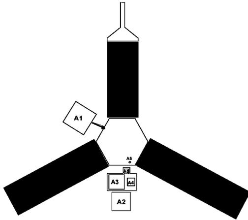
Figure 4. Juno Spacecraft with MWR Antenna locations shown.
