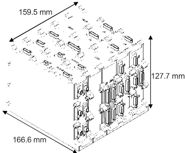
Figure 14. MWR EU Assembly with CBE Dimensions.
