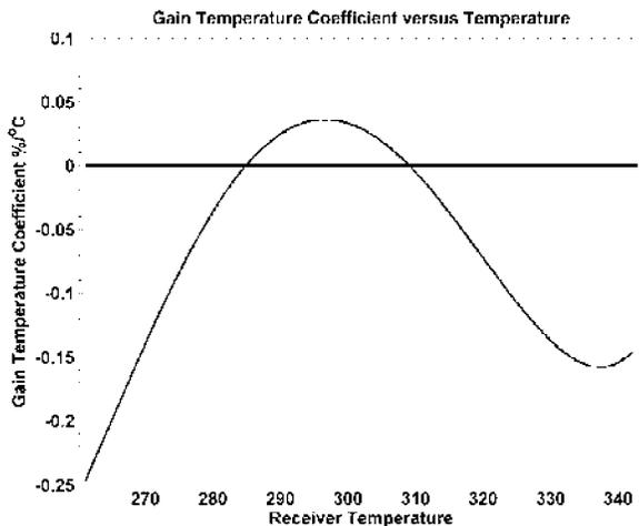
Figure 17. Temperature coefficient of R2 radiometer gain.
